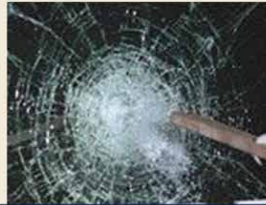
9 LB 2X4 MISSILE SHOT AT 50 FT/SEC TESTS IMPACT WINDOW
