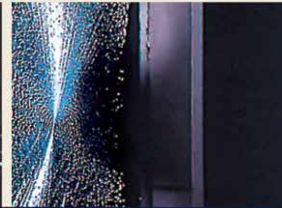
LAMINATED GLASS MAY CRACK UNDER PRESSURE, BUT TENDS TO REMAIN INTEGRAL, ADHERING TO THE VINYL INTERLAYER
